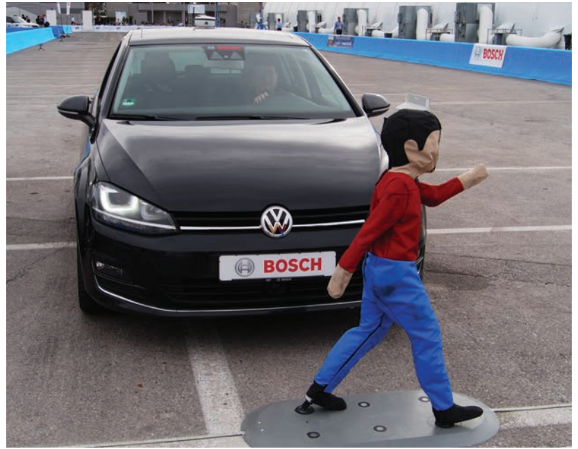
The Bosch Pedestrian Detection and Automatic Braking system in action; stereo cameras detect "Timmy" and apply brakes, autonomously bringing the car to a full stop.
